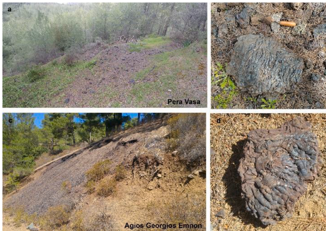
Fig. 4. a. The slag heap of Pera Vasa is hidden under a thick pine forest. b. Large slag cake from Pera Vasa slag heap. c. The slag heap of Agios Georgios Emnon. d. Large slag cake from Agios Georgios Emnon slag heap (Photographs V. Kassianidou).
