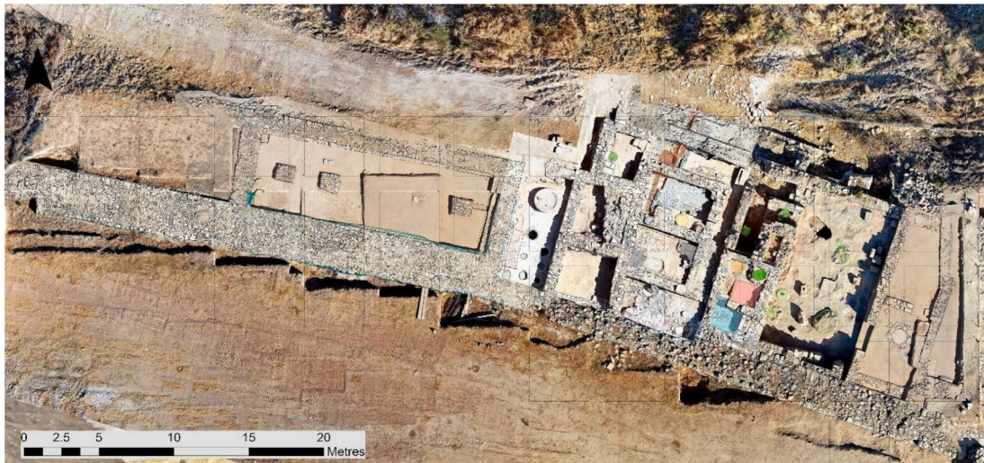
Fig. 5. True orthophoto mosaic over the Hadjiabdoulla workshop complex generated from photogrammetric structure from motion (SfM) processing of high-resolution low altitude nadir and oblique drone images. Vectors over the mosaic highlight archaeological findings and trenches (drafted by Athos Agapiou).
