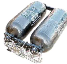
Hydrogen tanks used for on- board applications
