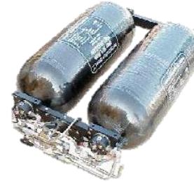
Hydrogen tanks used for on-board applications
