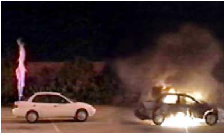
Fire in petrol engine (15,000 vehicle fires in GER/year) and the hydrogen vehicle (left) with leaking tank.
