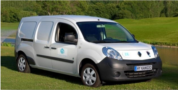
Renault HyKangoo: 300 km range, plug-in-battery with 5 kW range extender, ca. 200 pcs
