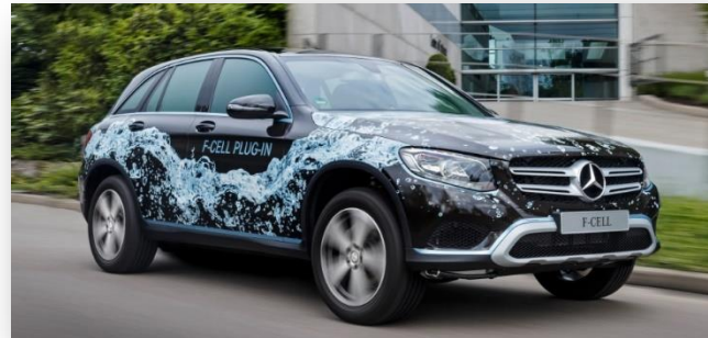
Mercedes GLC: starting 2019, fuel cell with plug-in-battery, 500 km range (50 km by battery)
